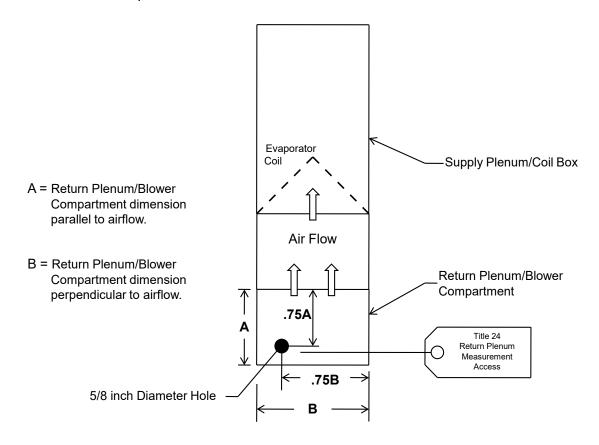
Figure RA3.2-1 Measurement Access Hole
