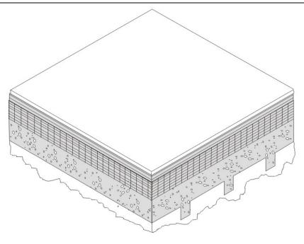
Figure 4.2.6 – Span Deck and Concrete Roof
