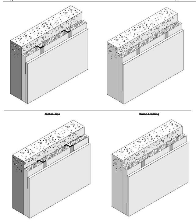
Figure 4.3.14 – Interior or Exterior Insulation Layers
