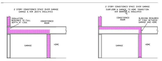
Figure RA3.5-9 Homes with Conditioned Space Over Garage – Structural Insulated Panel (SIP)
