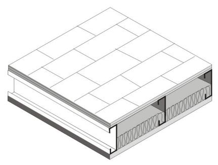
Figure 4.2.5 – Metal Framed Rafter Roof
