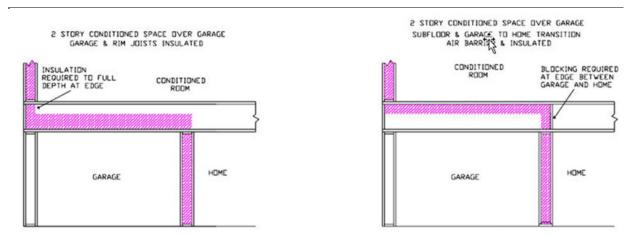
Figure RA3.5-11 Homes with Conditioned Space Over Garage – Insulated Concrete Form (ICF)
