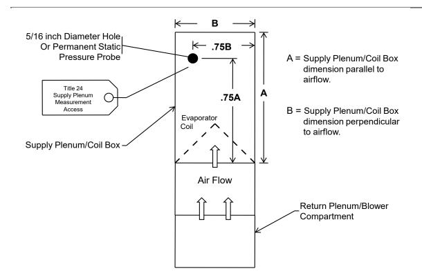
Figure RA3.3-1 Hole for the Placement of a Static Pressure Probe (HSPP) or Permanently Installed
