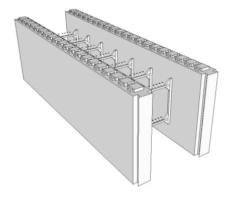
Figure 4.3.13 – Insulating Concrete Forms
