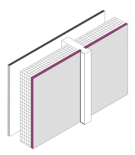
Figure 4.3.8 – Spandrel Panel
