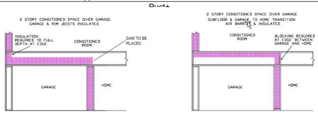
Figure RA3.5-3 Homes with Conditioned Space Over Garage – Loose Fill Insulation
