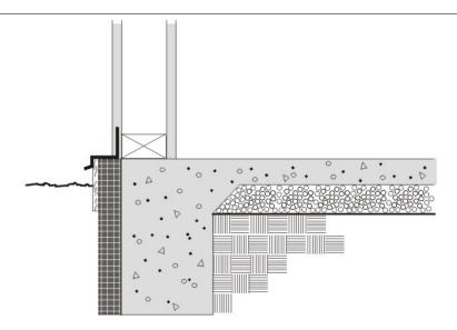
Figure 4.4.7 – Unheated Slab-on-Grade Floor
