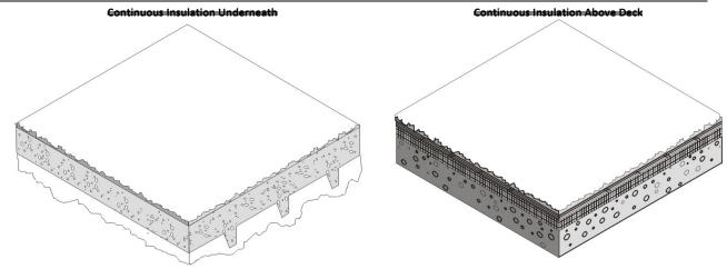
Figure 4.4.6 – Concrete Raised Floors
