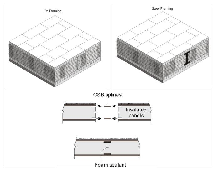
Figure 4.2.3 - SIPS Roof/Ceiling
