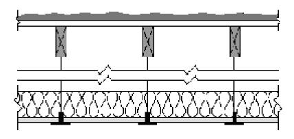
Figure 4.2.8 – Insulated Ceiling with Removable Panels
