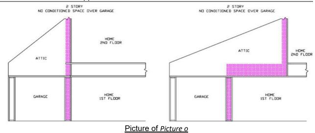
Figure RA3.5-6 Homes with No Conditioned Space Over Garage – Rigid Board Insulation
