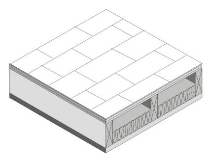
Figure 4.2.2 – Wood Frame Rafter Roof
