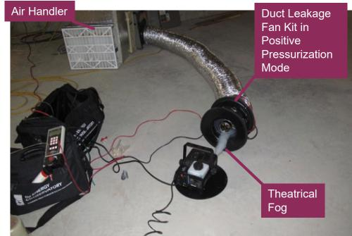
For existing altered ducts unable to meet the Total Duct Leakage or Leakage to Outside tests, a Smoke Test and Visual Inspection can be used:
