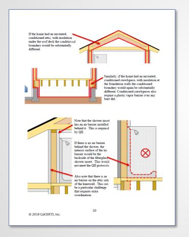
Tub and shower inserts on an exterior wall, must have air barrier behind them.
