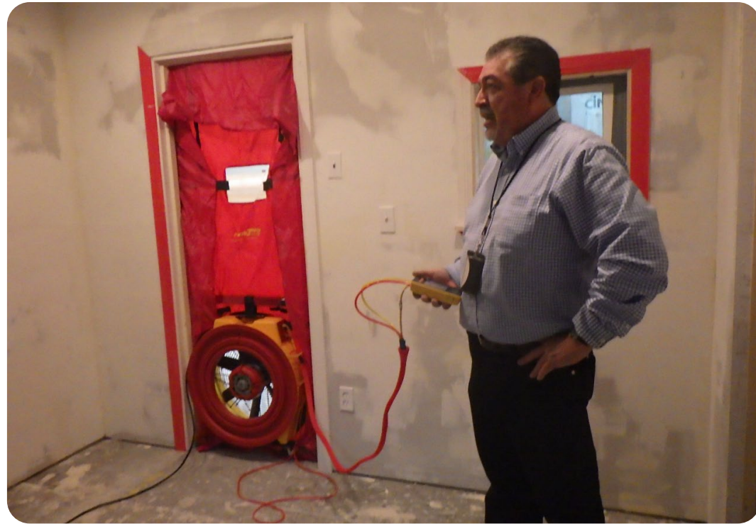
3C-REN instructor Javier Saucedo demonstrates blower door testing
